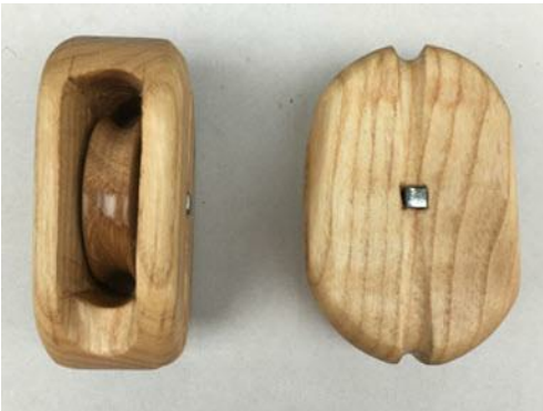
Finished blocks with sheaves in place.
