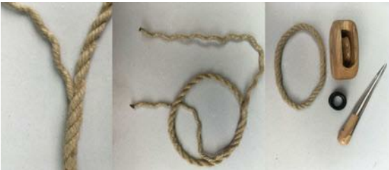
Creating a strop. L-R removing one strand from the rope, laying up the grommet, the finished article.
