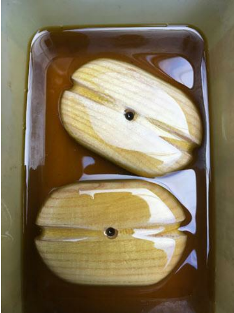
Finished shells soaking in linseed oil.
