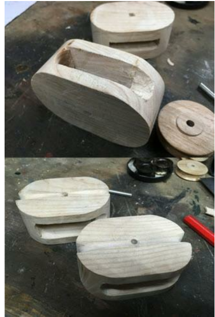
Morticed shells cut to shape.
