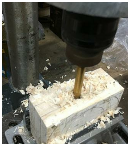
Morticing the shell on the pillar drill.
