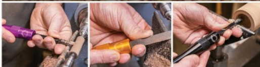
M.R. Each handle has a 7.5mm bore with twin grub screws to secure the blades in place.
