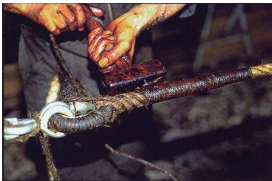
Serving a very tarry eye splice Graham Machlachlan, Knotting Matters Issue 78, International Guild of Knot Tyers, March 2003
