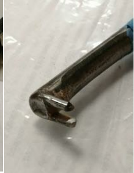
Hollowing tool based on the Melvyn Firmager hollower.
