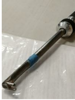
Hollowing tool based on the Melvyn Firmager hollower.
