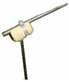
Diagram 2: Sharpening Jig. Copyright © Andrew Lodge. Reproduced with permission.
