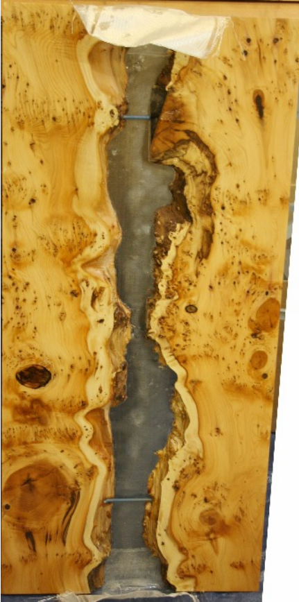
Above - Small plank, cut in half and re-joined with steel spacers. No resin yet.
